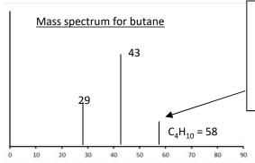
The peak with the highest mass/charge ratio will be normally due to the original molecule that hasn't fragmented (called the molecular ion). As the charge of the ion is +1 the mass/ charge ratio is equal to Mr.
