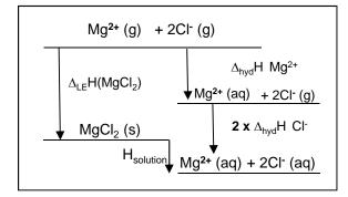
When an ionic substance dissolves the lattice must be broken up. The enthalpy of lattice dissociation is equal to the energy needed to break up the lattice (to gaseous ions). This step is **endothermic.**
