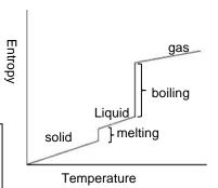
At 0K substances have zero entropy. There is no disorder as particles are stationary
