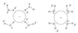
The higher the **charge density** the greater the hydration enthalpy (e.g. **smaller ions** or **ions with larger charges**) as the ions attract the water molecules more strongly.
