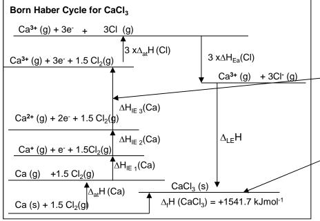
The big increase in ionisation enthalpy to remove the 3rd electron is not compensated for by the stronger lattice enthalpy of formation
