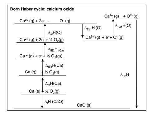
Notice the second electron affinity for oxygen is **endothermic** because it take energy to overcome the **repulsive force** between the **negative ion and the electron**
