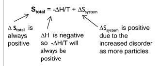
For salts where H solution is endothermic the salt may dissolve depending on whether the **S** value is more positive than - H/T is negative
