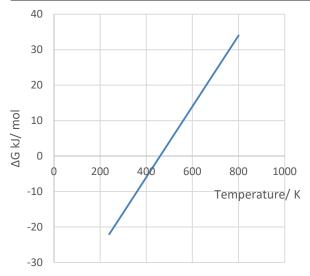
The slope of the line would change below 240K because ammonia would be a liquid and the entropy change would be different
